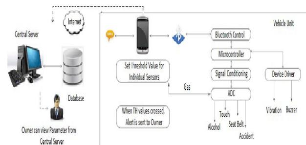
This system is an intelligent vehicle monitoring system which consists of a real time monitoring smart vehicle unit. The system is integrated with GPS and Bluetooth Connectivity to provide real time tracking using SMS, real time monitoring sensors. The main components of the system consist of number of real time sensors like:
